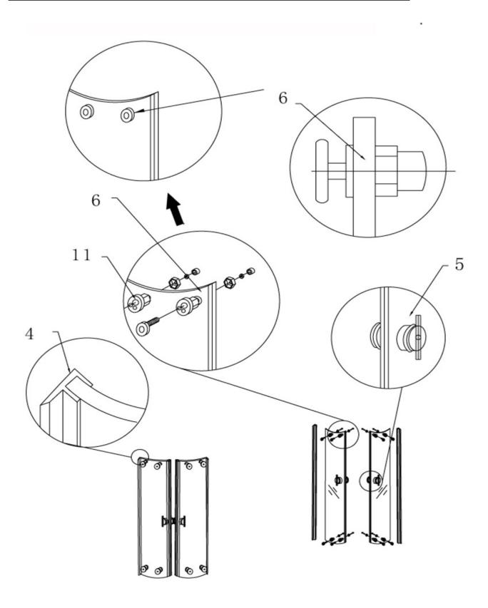
**6. Glass Door Installation** Install glass door to the rails as shown by the illustration.
