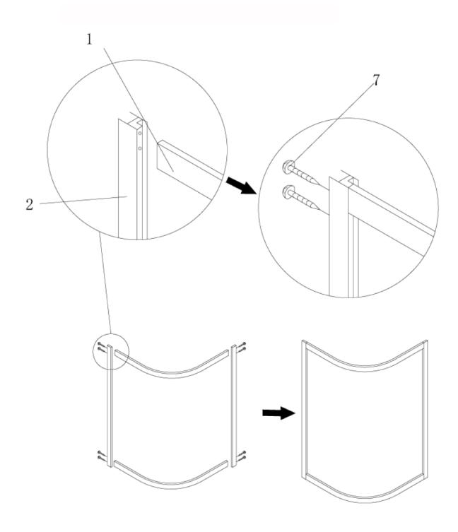
**4. Glass Panel Installation**Install fixed glass panels to the door frame as shown by the illustration.
