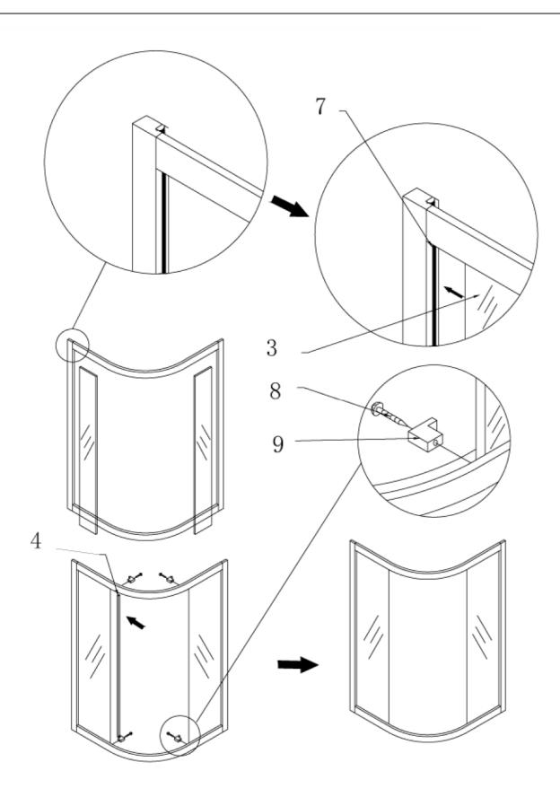
**5. Glass Door Assembly** Install door rollers and water seal strips as shown by the illustration.
